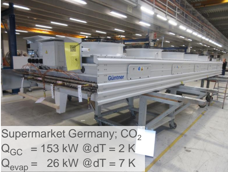
Supermarket Germany; CO 2 Q_{GC} = 43 \text{ kW @d}T = 2 \text{ K} Q_{\text{evap}} = 25 \text{ kW @d}T = 7 \text{ K}
